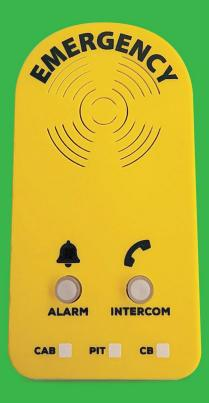
The device enables two-way voice communication from the lift cabin to the service centre and to the mobile phones of the emergency service crew. In cooperation with the centre, it provides the required connection and battery capacity checks. The LEMON device from the BC production can be used as the centre or it can be connected to a centre using the P100 protocol. The Kk-CEMOL device can also be used for data transmission in cooperation with the LEMON centre.
